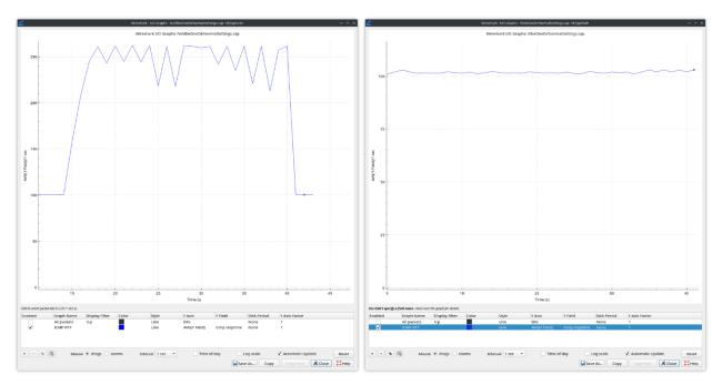
As you can see, the latency experienced by the ping test on the link jumped significantly to around 250mS when ViBE is not in use (left graph,) whilst remaining completely unaffected at just over 100mS when it is (right.)
