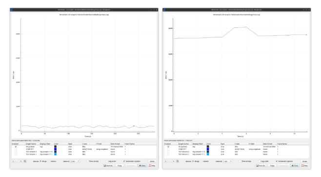
Here you can see a huge difference, with the non-accelerated transfer taking around 25 times longer to transfer this 100 megabyte file. As has been mentioned, a loss figure of 1% is not that uncommon, especially when you consider that such an event may only happen for a few seconds at a time, briefly killing any transfers in progress when it does and causing a recovery period when it returns to normal.
